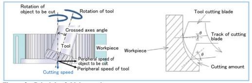
Figure 3 Principle of skiving cutting
