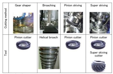
Figure 2 Gear cutting method of internal gear
