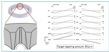
Figure 11 Tooth lead accuracy in tapering cutting
