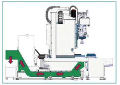
Figure 5 Center trough structure
