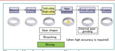
Figure 1 Manufacturing process of internal gear
