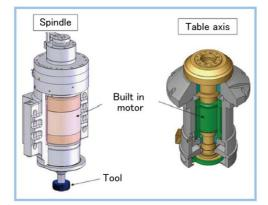
Figure 7 Structure of spindle and table axis
